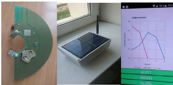
Fig. 2. Appearance of the sensor, hub and graphs on a smartphone.
