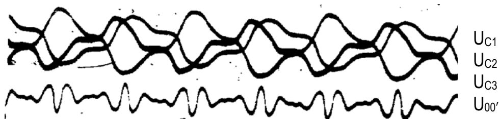
Fig. 5. Oscillograms of the voltage in the capacitor of the SHC \left(\frac{\Omega}{3}\right) in a three-phase EFMC.
