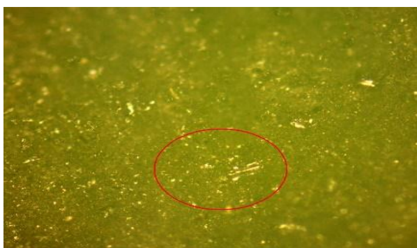
Figure: 4. Coal surface of the Angren-1 mining site at tenfold magnification on a polarizing microscope AXIOScope A1 of the German company ZEISS.
