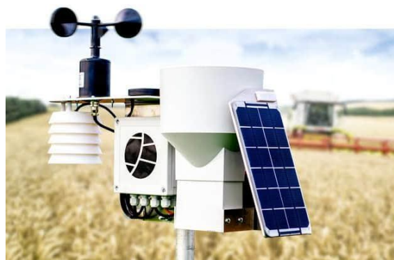
Figure 4. Device for monitoring solar and wind characteristics
