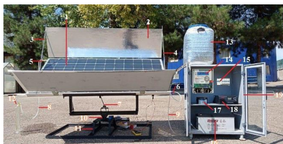
Fig. 3. Photo thermal installation based on a photo thermal battery of a new design.
