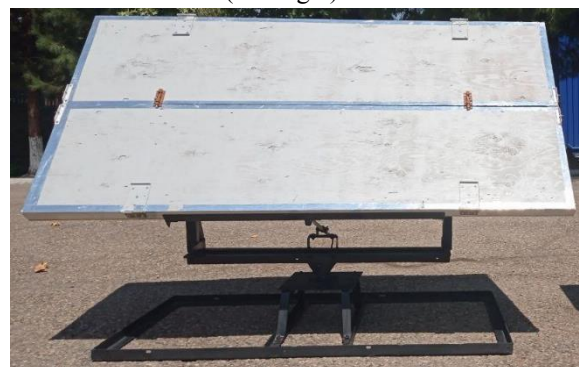
Fig. 4. Photo thermal battery after measuring parameters in natural conditions.
