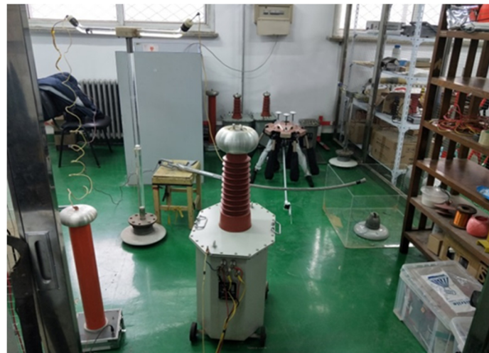
Fig9. Safety distance test platform
