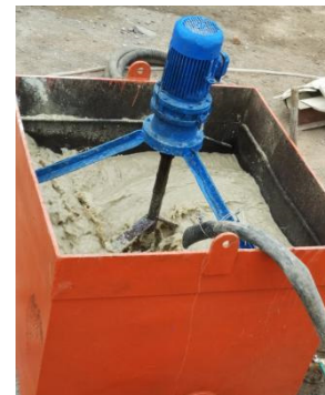
Fig.5 preparation of test slurry
