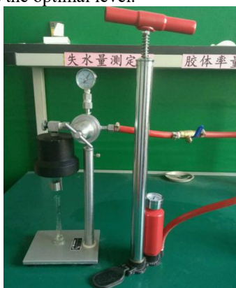
Fig.3 test of slurry water loss
