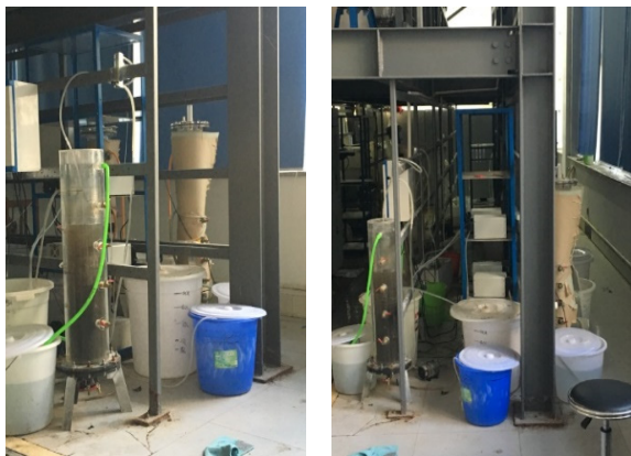
Fig3. Device diagram of SBBR-UASB reactor
