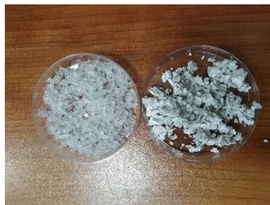
Fig. 2. Samples of waste polymer components EVA and Tedlar® of polycrystalline solar panels.
