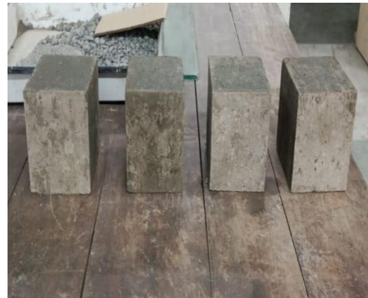
Fig. 10. Concrete blocks left for air drying.
