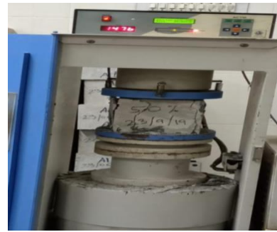
Fig. 9. Compressive Strength Test using Compression Machine.
