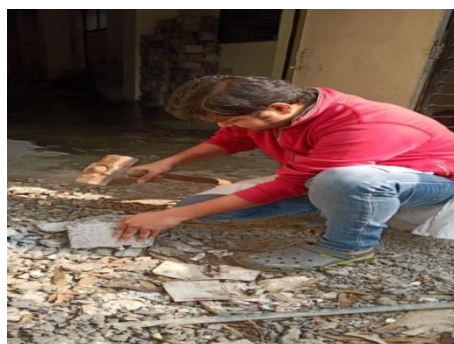
Fig. 4. Crushing of Concrete Cubes using Hammer.
