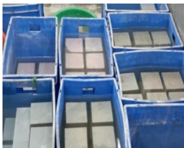
Fig. 7. Curing of concrete cubes.
