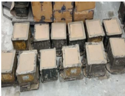
Fig. 6. Casting of concrete cubes of size 150 mm.
