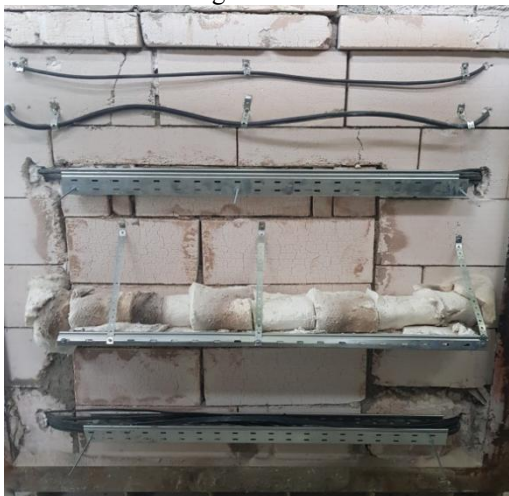
Fig. 6. Mounted cable samples and schematic section on the test furnace wall.
