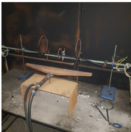
Fig. 2. Appearance of the cable sample VVGng(A) - FRLS 3*10 before the tests.
