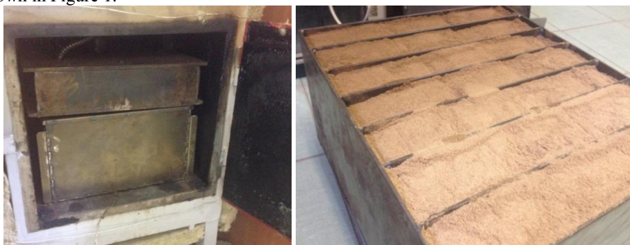
Fig. 1. Experimental unit for thermal modification of crushed wood in a dense bed.
