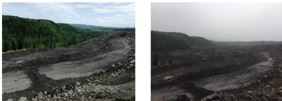
Fig. 1. Photo of the Kiyzassky open pit stockpile before the landslide (left) and after the landslide (right)
