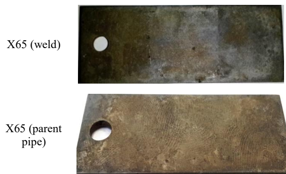
Fig. 3. View of steel samples after testing under conditions of moisture condensation in the presence of CO 2 [14].
