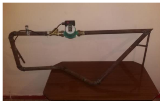
Fig.1. Installation for investigation of corrosion in internal compartments of steel pipes.
