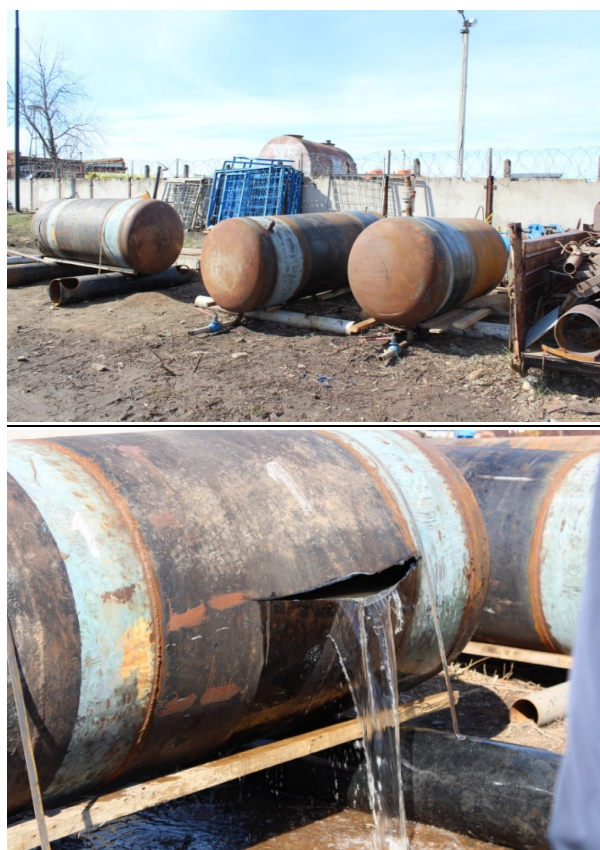
Fig. 6. Sample barrels before and after hydraulic testing.
