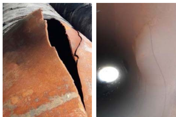
Fig. 1. Defects in the form of delamination detected after testing a full-size pipe with internal blistering.
