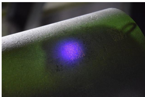
Fig. 3. FDPM on a steel pipe after shot blasting, photo in fluorescent light.
