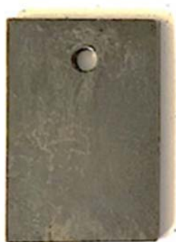
Fig. 2. View of sample after conducting autoclave testing in conditions approximate to real-life (20% NaCl, pH 3.5, 175°C, P H 2 S = 3.5 MPa, P CO 2 = 3.5 MPa).
