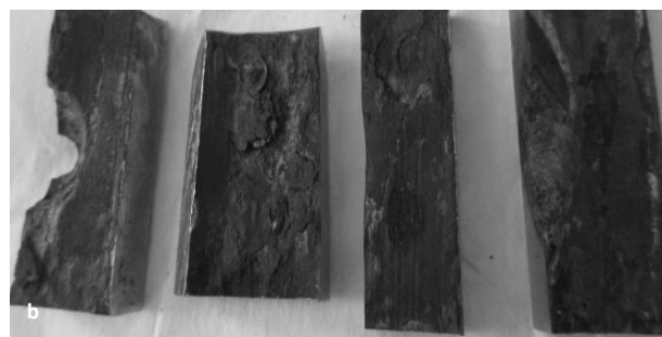
Fig. 2 Exterior view of the inner surface on the samples: a) after 244 days of operation with high levels of CANI and NMI, b) after 344 days of operation with low levels of CANI and NMI.
