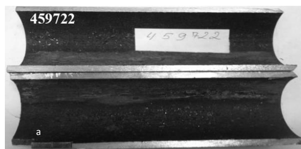
Fig. 3 The results of metallographic examination of corrosion products a) on tubing corresponding to GOST 633 (chromium-free), b) on tubing made of chromium-containing steel grades.
