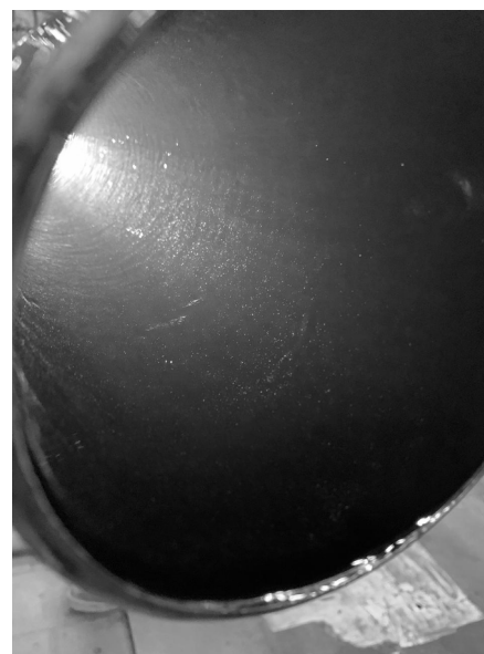
Fig. 2. An inner surface of a pipe coated with KronEpur 80.
