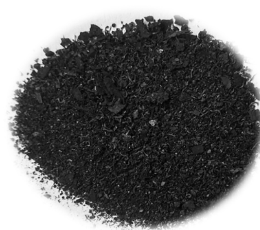
Fig. 4. The appearance of the sediments from the tar.
