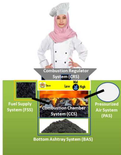
Fig. 1. Concept design of Hi-Tech Cook Stove (HTCS)
