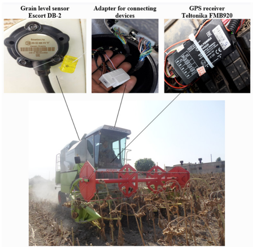
Fig. 2. Outlook of the adapted combine harvester equipped with GPS receiver, grain sensor.
