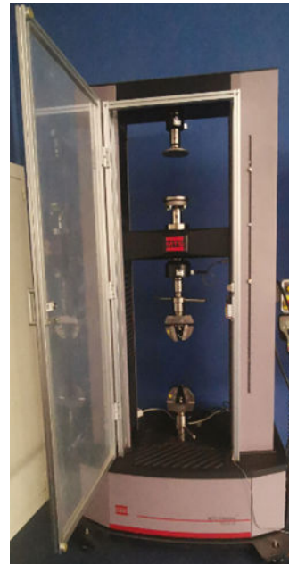
Figure 1: MTS series 40 machine used in the experimental test.
