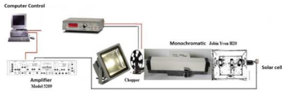
Figure 1. Measuring bench (IPCE) for measurements of the external quantum efficiency (QE).
