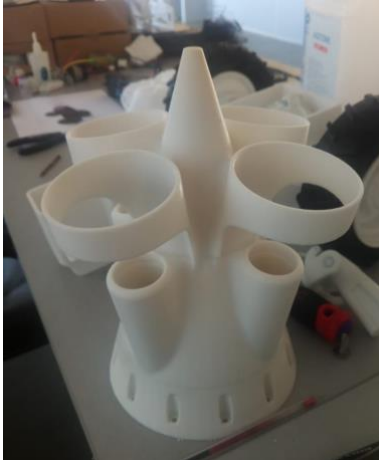
Figure 8: ROV's stern in 3D prototyping
