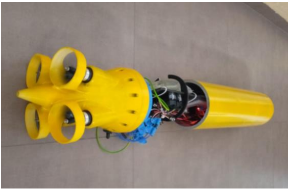
Figure 9: ROV's assembly in progress
