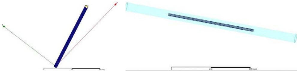
Fig. 4. Design model of antenna and material (hydrate) to be heated.
