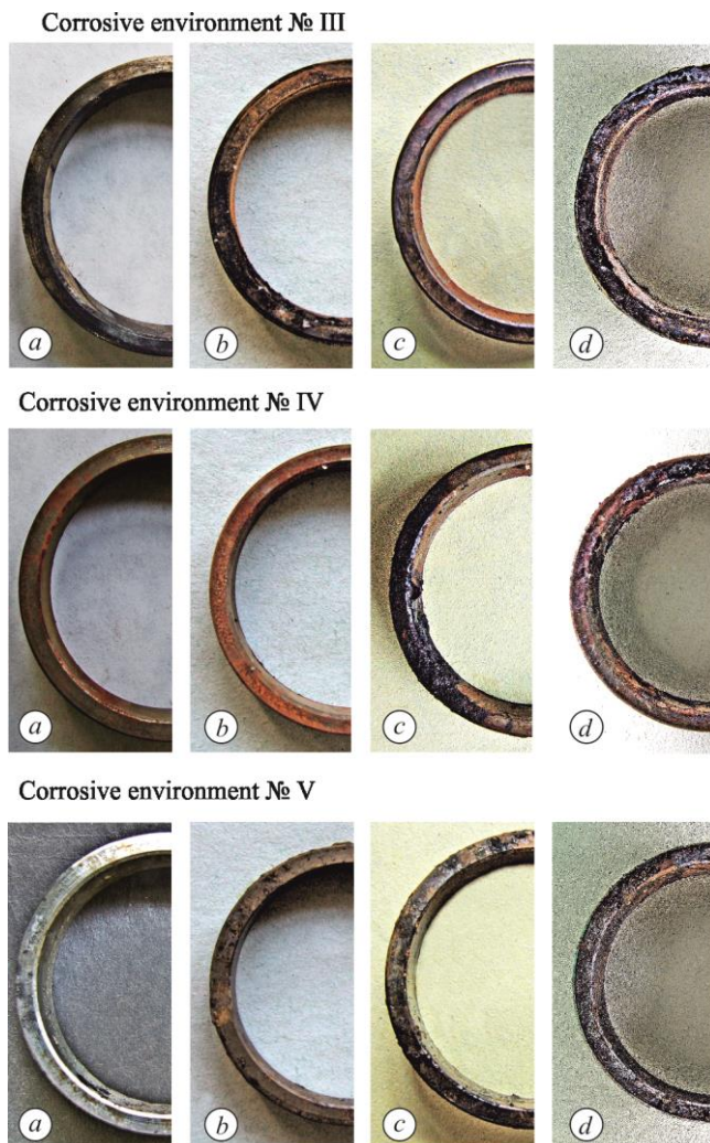
Fig. 6. The surface of the samples after exposure in the neutral solutions (III, IV, V) duration 24 h (a), 168 h (b), 288 h (c), and 576 h (d).
