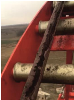
Fig. 1. Corrosion damage to the CT pipe after acid jobs.
