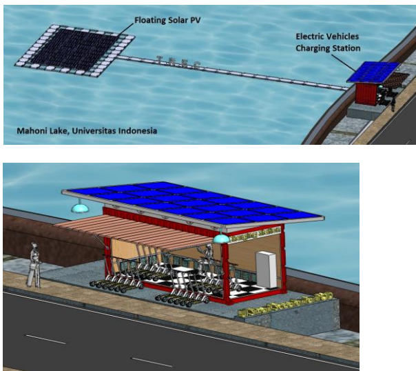
Fig. 6. Electric Vehicles Floating PV Charging Station
