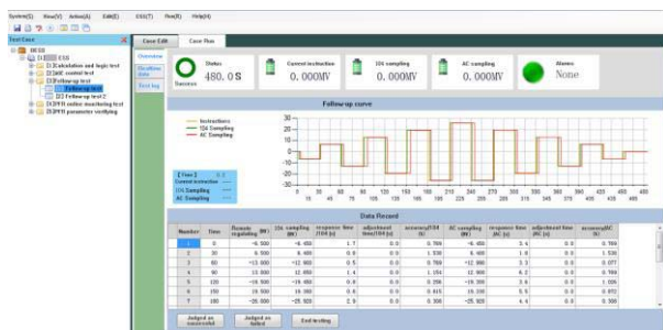
Figure 6 AGC follow-up test interface of simulation and test system for energy storage station
