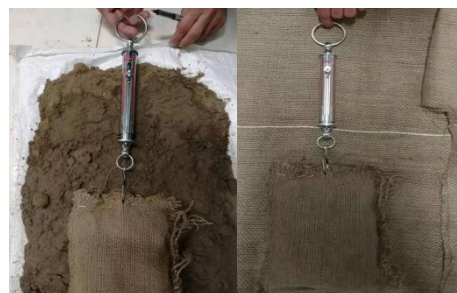
Fig 5. Friction coefficient measured of jute ecological bag
