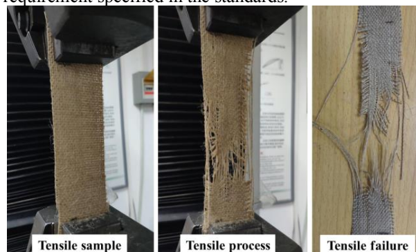
Fig 2. Tensile sample of jute cloth before and after tensile failure
