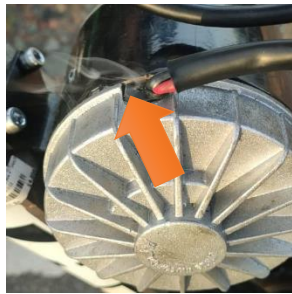
Fig. 13. Motor burn out as a result of experimental test.
