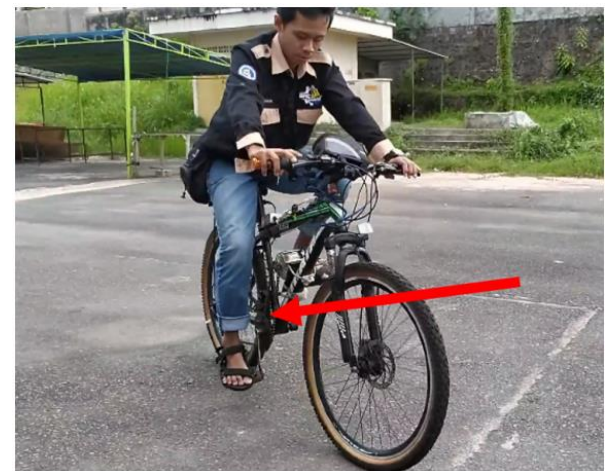
Fig. 10. Motor help rider to pull front wheel to make ebike move.
