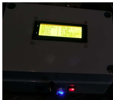
Figure 6. Display of water quality and battery voltage monitoring on the LCD.
