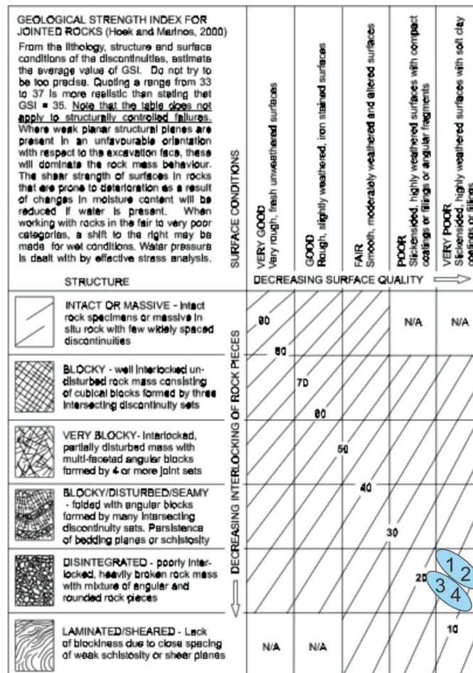
Fig. 4. GSI estimates from the geological face mapping observation on GSI chart [13].
