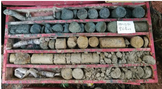
Fig. 5. Core drill zone 1 at 30-35 m depth (documentation of PT. KCIC)
