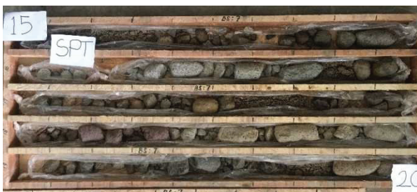
Fig. 6. Typical drill cores at the research location, material lapilli tuff poor quality
