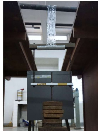
Fig. 3. Geocell connection test (blind rivet).
