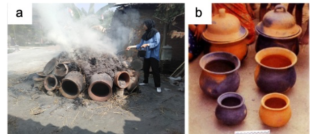
Fig. 3. a. Traditional firing system in Ndolon. b. Ceramic products with open firing systems [9].
