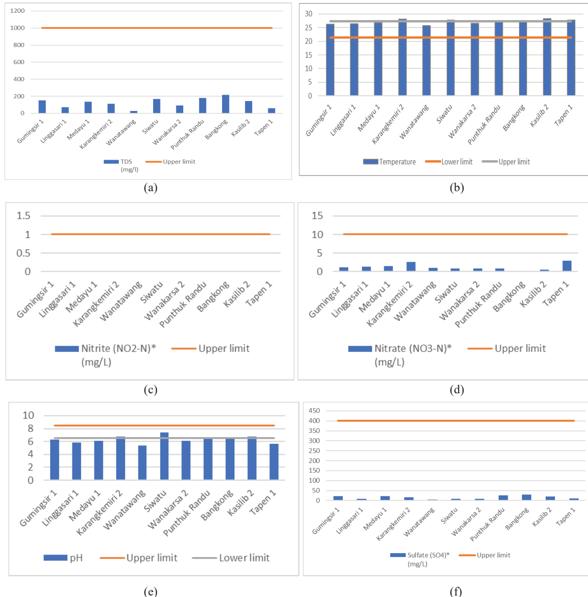
Fig. 3. Charts of the water quality test results and standards for sanitation and hygiene purposes: (a) TDS, (b) temperature, (c) nitrite content, (d) nitrate content, (e) pH and (f) sulphate
