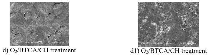
Fig. 2. SEM images of chrome tanned leather with 100x (left) and 2000x (right) magnifications: a, a1) untreated; b, b1) O 2 plasma pretreated; c, c1) O 2 /BTCA treatment and d, d1) O 2 /BTCA/CH treatment
