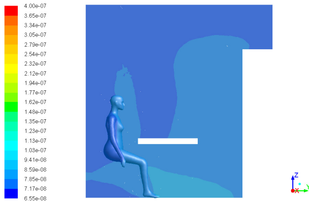
Fig. 9. Mass fraction of pollutant UDS3 [kg/kg] in a vertical mid-plane through the mannequin
