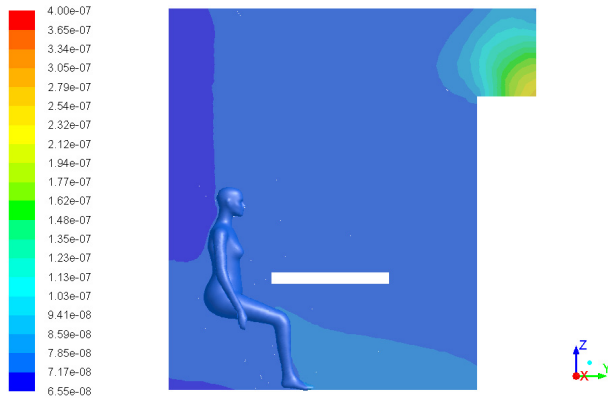
Fig. 10. Mass fraction of pollutant UDS4 [kg/kg] in a vertical mid-plane through the mannequin
