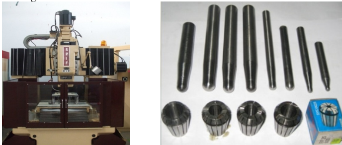
Fig. 4: a. Specialized SPIF machine of DCSELAB; b. Self-manufactured tools and standard bores collets
