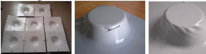
Fig. 7: PVC model are formed to get torn lines or failures to reach a biggest angle of deformation [6]
