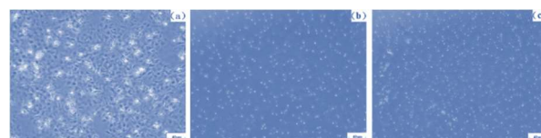
Fig 4. Physical appearances of (a): saturates, (b): saturates+500 mg/kg EVA and (c): saturates+500 mg/kg PPD
