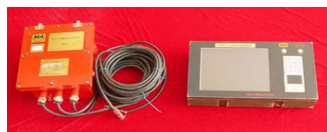
Fig.6 Wireless measuring system (outside hole part)
