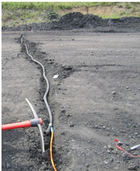
Fig. 2. Laying an electrical prospecting streamer across the technological road.
