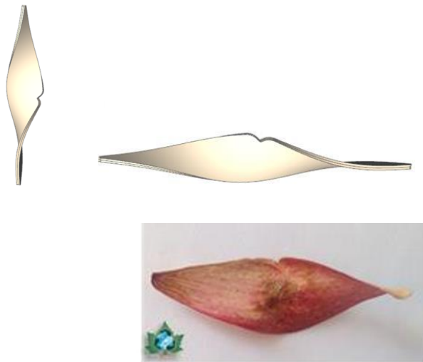
Fig. 8. The bioengineering model of the Rhus typhina seed used as model for blades and paddles
