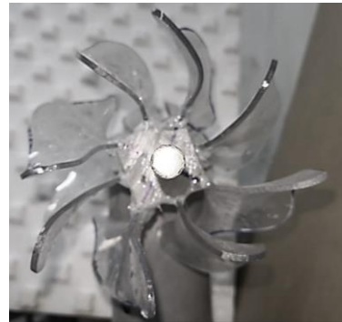
Fig. 12. The axis with 8 paddles in the shape of a Rhus typhina seed. Longitudinal view, detail and cross-sectional view
