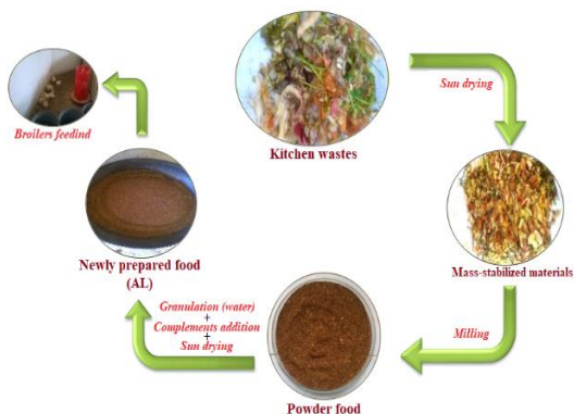
Fig. 2. Lab manufacturing steps of the lab-prepared food (LPF)
