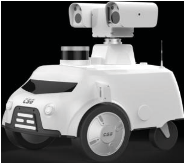
Fig. 1. Appearance of wheeled inspection robot
