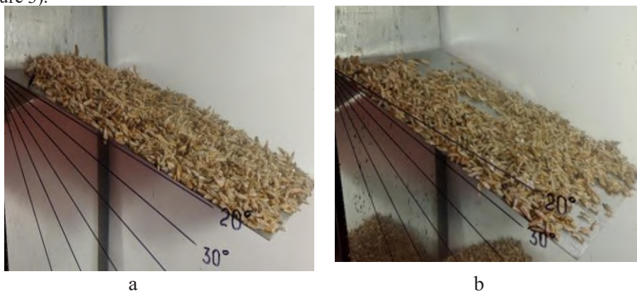
Fig. 3. General view of grains immersed on the surface of an inclined plate with an installation angle \alpha = 20^\circ (a) and \alpha = 30^\circ (b) to the horizon when grain is fed by a stream from a height of h = 0.050 m.
