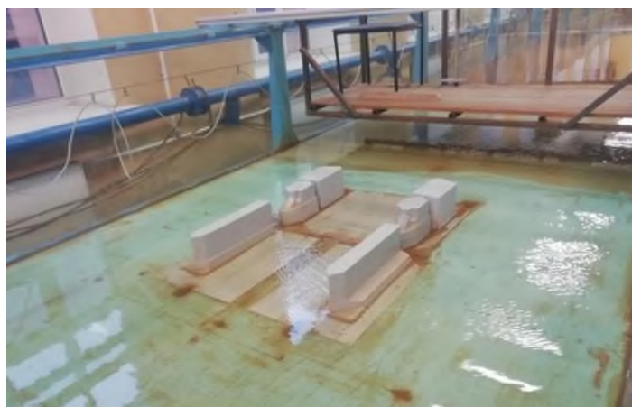
Fig. 1. The location of the supports of the existing and designed bridges in the hydraulic flume.
